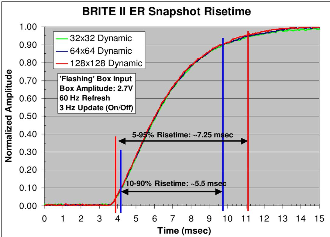
Figure 5 – BRITE II ER Emitter Array Risetime Measurement (Snapshot Mode)
