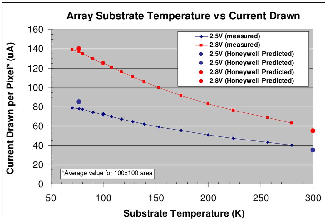
Figure 10 – BRITE II ER Array Cryogenic Operation Performance
