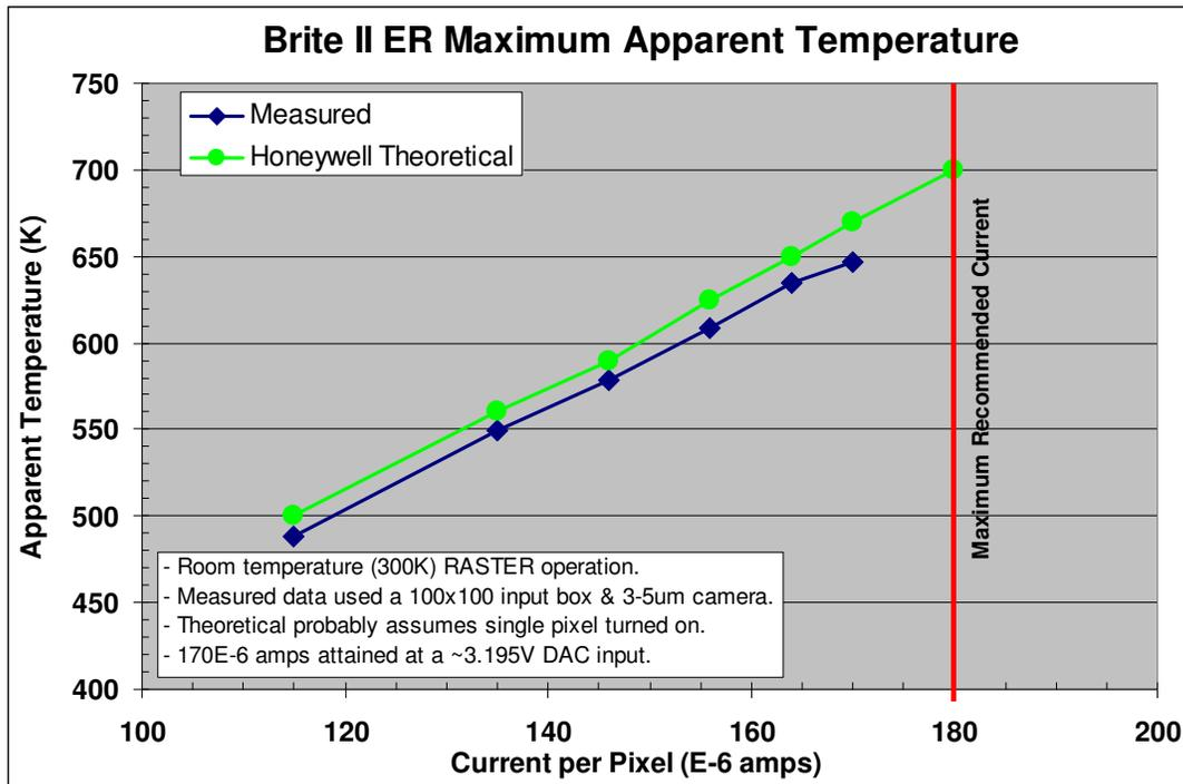
Figure 6 – BRITE II ER Array Maximum Apparent Temperature
