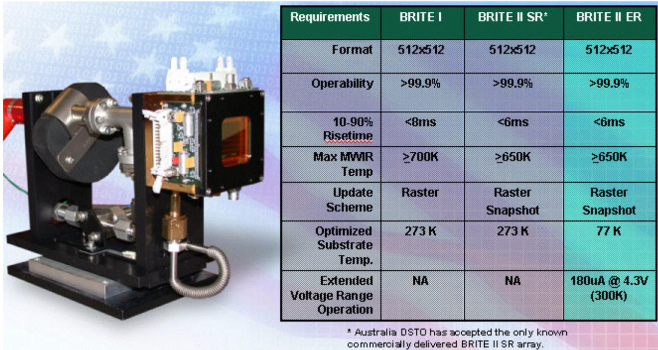
Figure 2 – BRITE II SR and ER Array Requirements
