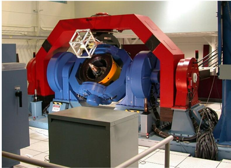
**Figure 12 – FMS Table in the AMRDEC ASC**
