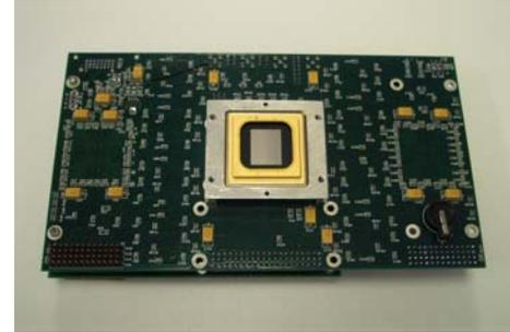
Figure 6 : XGA Drive Electronics Board
