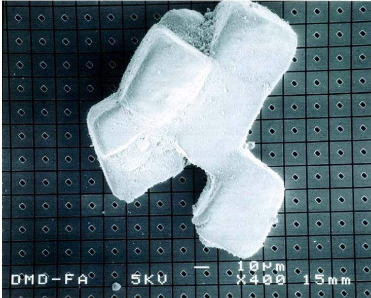
Figure 2: DMD with Grain of Salt on Surface
