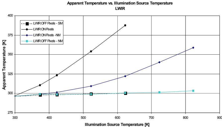
Figure 18: LWIR Apparent Temperature vs. Illumination Source Temperature
