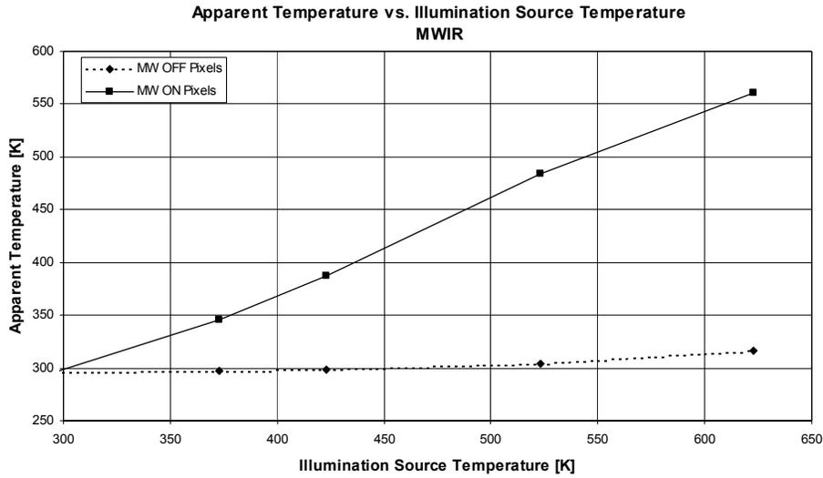
Figure 17: MWIR Apparent Temperature vs. Illumination Source Temperature
