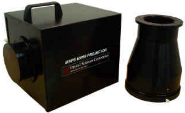
Figure 11 – IR-MAPS Projector With Dual Collimators
