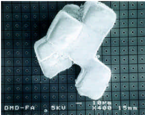
Figure 2: DMD with Grain of Salt on Surface
