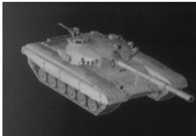
Figure 19: LWIR SVGA Collected by 320x240 Uncooled Bolometer Array Camera
