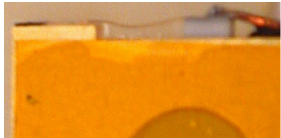
Figure 10: Insufficient Bond Wire Clearance
