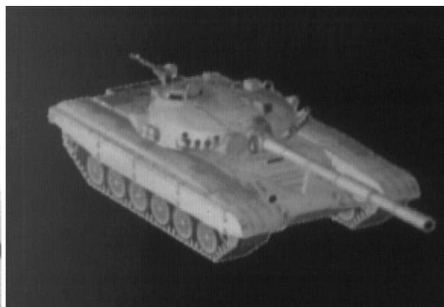
Figure 12: LWIR SVGA Collected by 320x240 Uncooled Bolometer Array Camera
