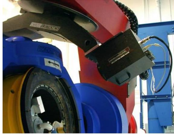
Figure 13: FMS-mounted MWIR projector
