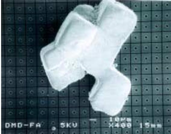
Figure 2: DMD with Grain of Salt on Surface
