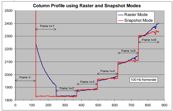
Figure 4: Comparison of MSSP Raster and Snaphot Update Mechanisms
