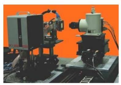
Figure 12 – Emitter array non-uniformity correction and characterization station
