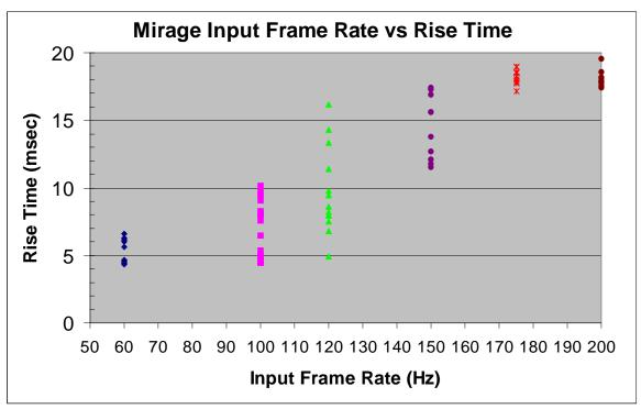
Figure 14: MIRAGE Overdrive Risetime Measurements
