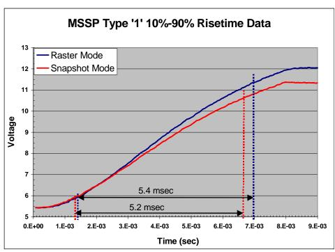
Figure 3: MSSP Raster and Snapshot Risetime Values
