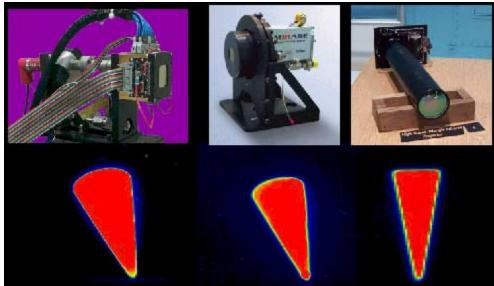
Figure 2: Dynamic IRSP Technologies and Example 'RV' Imagery
